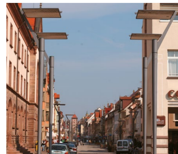
The FARO luminaires – very prominent luminaires in the cityscape. The existing luminaires were also retrofitted with LED.
